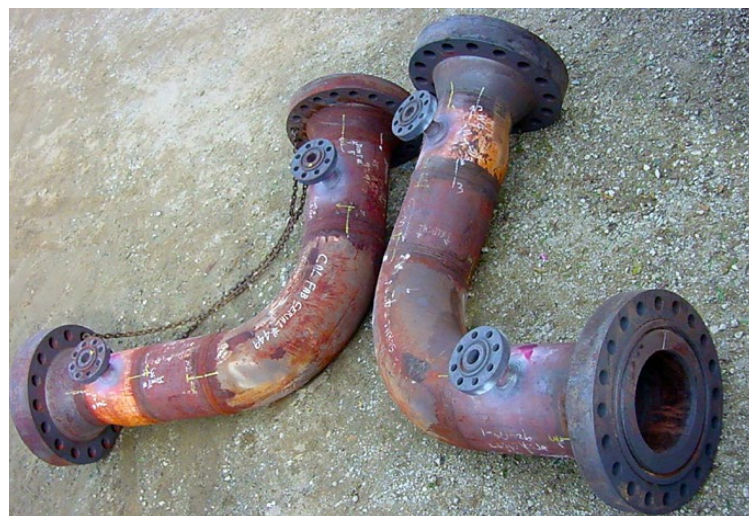
FIGURE 3. Elbows, like those pictured, can be used at offshore oil pumping stations. (Source: Fluid Components International)
