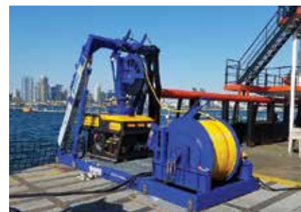
The surface dispersant monitoring launch and recovery system
