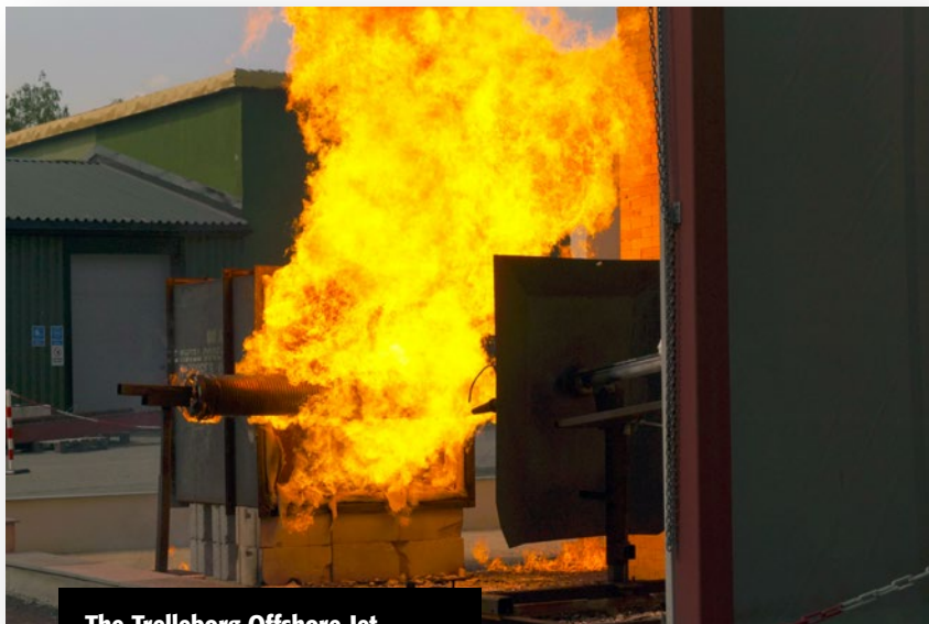
The Trelleborg Offshore Jet Fire test rig undergoes material qualification testing in Norway. (Source: Trelleborg Offshore)
