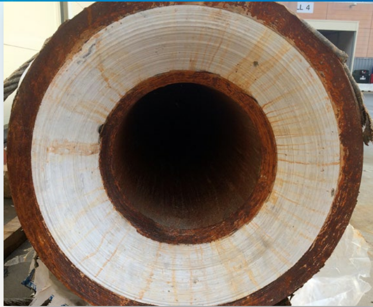
FIGURE 2. The conductor after a cut-and-pull operation with MOST Plus is shown. (Source: Weatherford)
