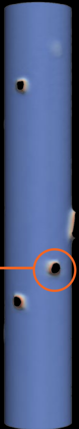
High Resolution 3D Images of Post-Fracture Perforations
