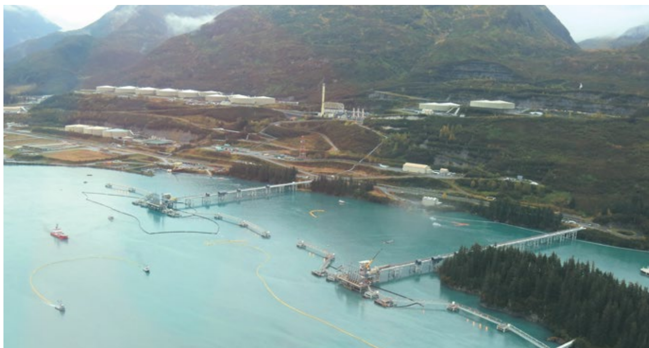
Port workboats set booms around tankers during loading at the Valdez, Alaska, pipeline terminal as a precaution in case of a spill. Source: Alyeska Pipeline Service Co.
