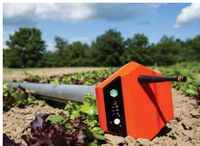
The soil probes from Teralytic can continuously measure phosphorus, potassium, carbon and other nutrients in soil and remotely communicate that data at 15-minute intervals for nature-based carbon offset projects.
