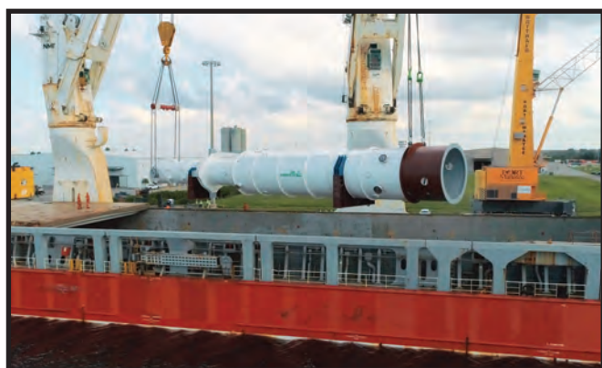
A completed LNG heat exchanger manufactured at Air Products' Port Manatee, Fla., facility is being loaded on a carrier at the Port of Manatee for shipment to the customer. (Source: Air Products)
