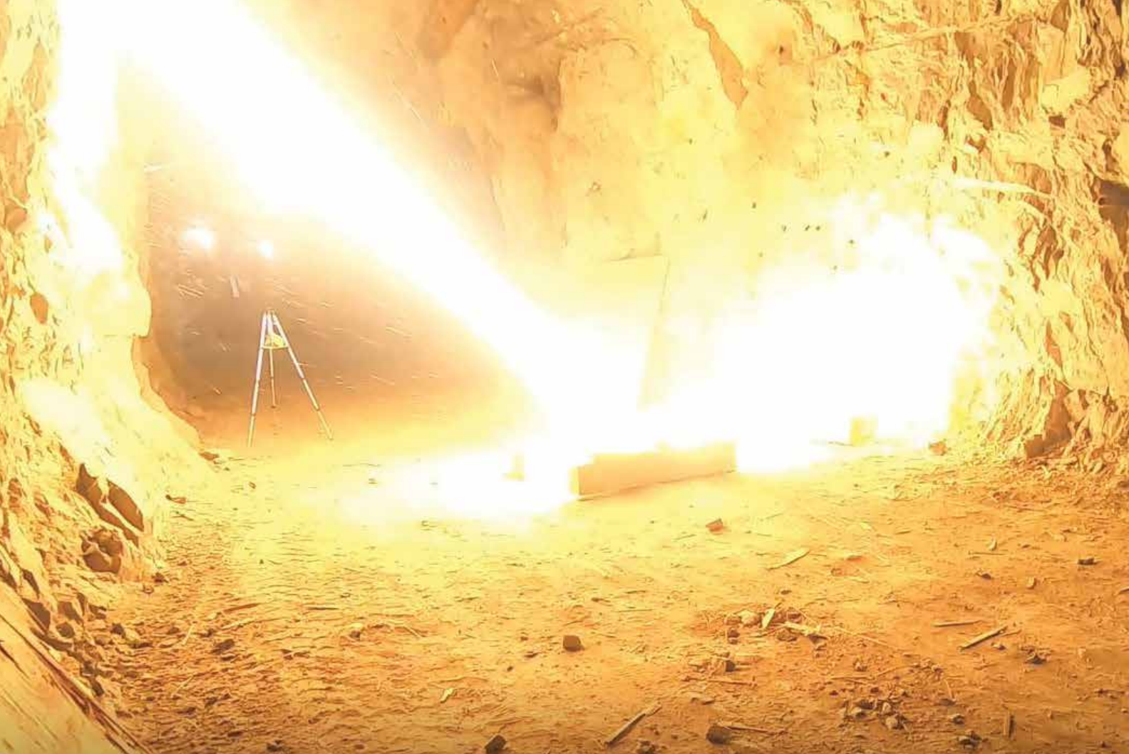
At the University of Texas at Austin, researchers in the Petroleum and Geosystems Engineering department are testing how a geometric cluster design, in which all clusters contain the same number of perforations, works in a naturally fractured reservoir.
