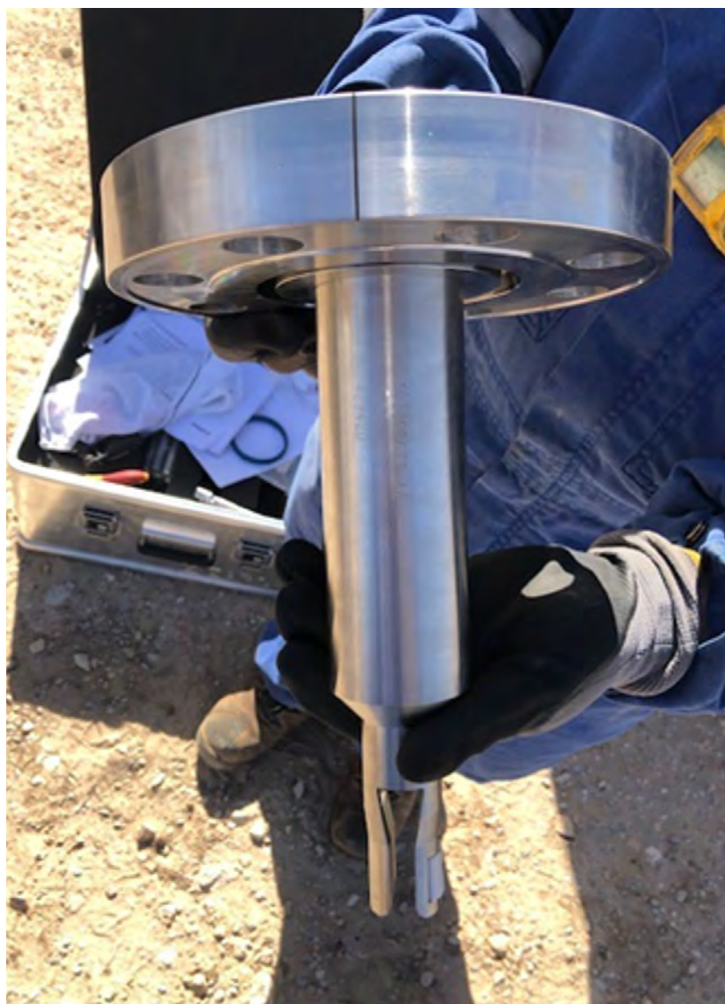
FIGURE 1. The low-rate extender insert is installed across the venturi section of a multiphase surface flowmeter. (Source: Schlumberger)
