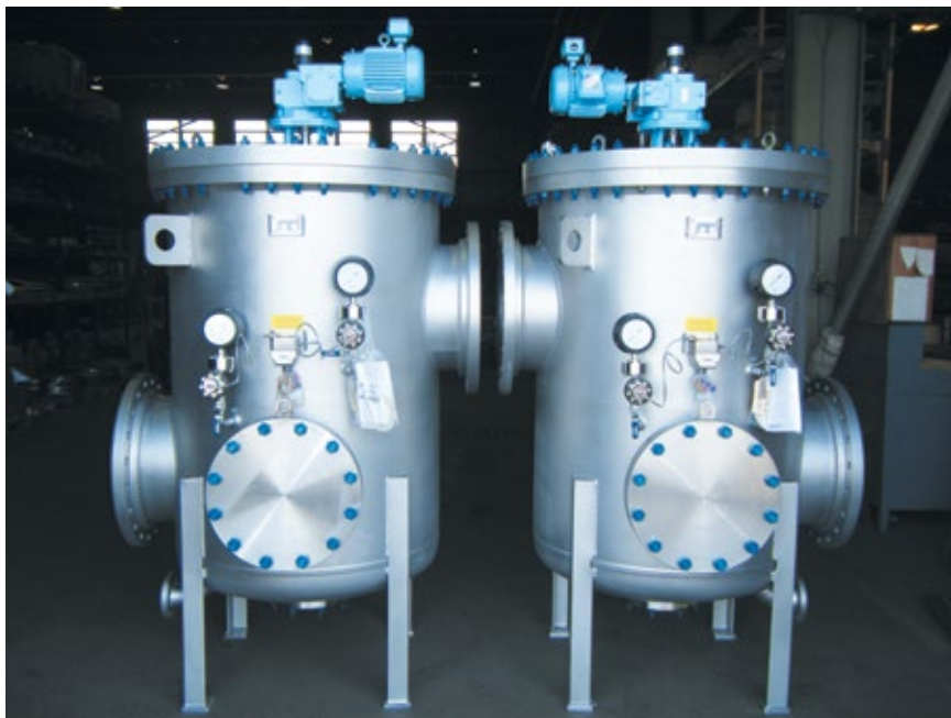
Rugged, well-engineered filter elements are designed to be cleaned in place by backwashing. Many installations have experienced an element life of more than 25 years. Source: R.P. Adams Inc.
