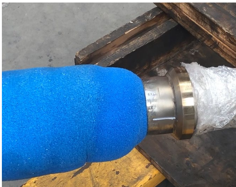
Filtrex is shown expanding out of a compression sleeve. (Source: Tendeka)
