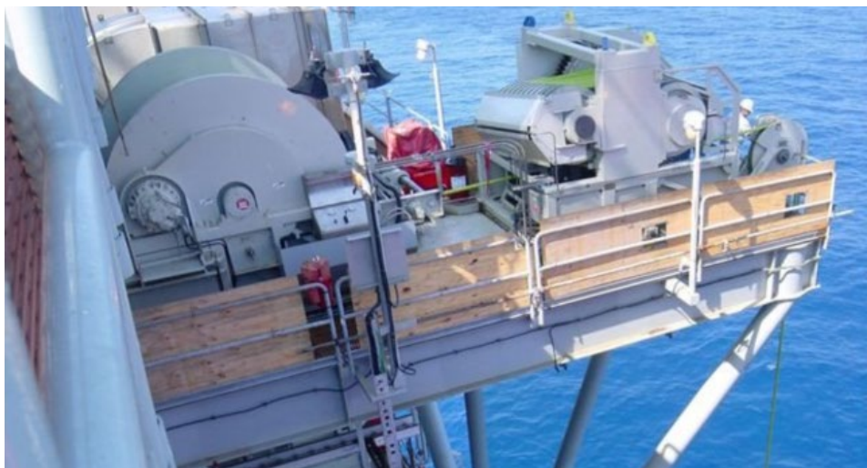
An offshore compensated coiled tubing lift frame was first deployed on the Atwood Condor. (Source: Logan Industries)
