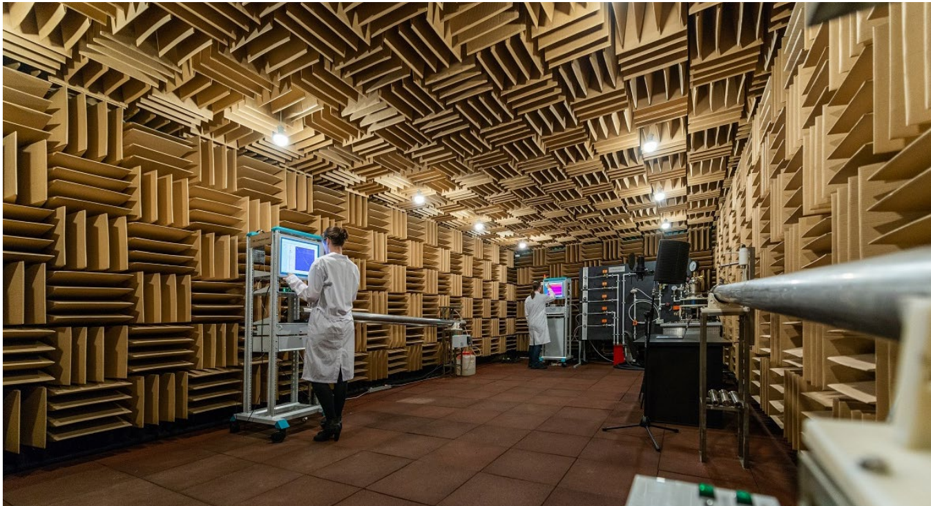
TGT's anechoic chamber completely absorbs reflections of sound waves, enhancing the company's acoustic diagnostic capabilities. (Source: TGT)
