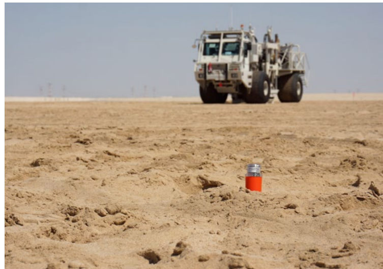
A 2019 trial of STRYDE technology in the United Arab Emirates set a new world record for land seismic trace density—184 million traces per kilometer. (Source: STRYDE)
