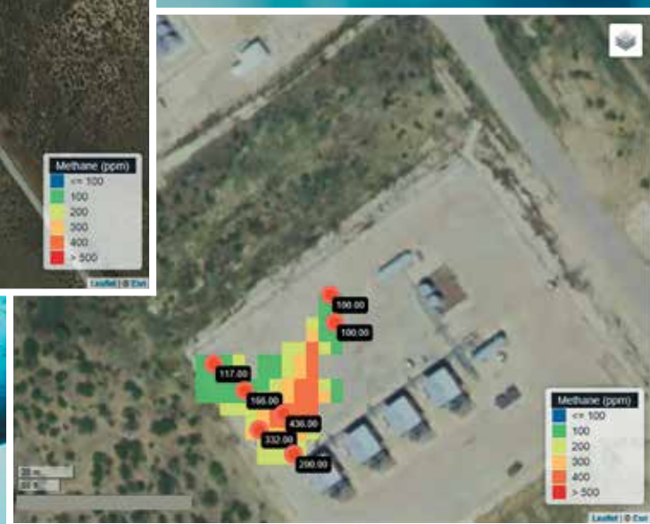
Satellite imagery plots the location and intensity of methane leaks around a Texas compressor station. Source: Satelytics
