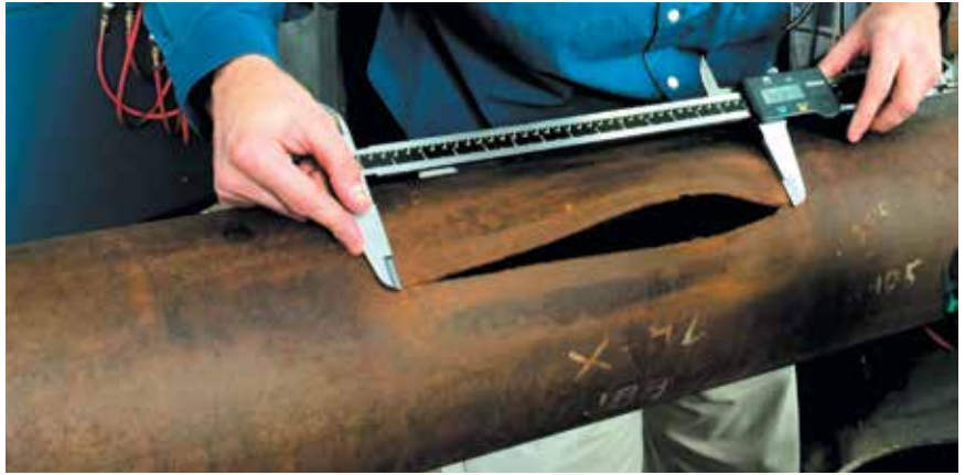
Critical crack/wall-loss models help inspectors detect flaws that could fail a pressure/hydro test. A new GTI model enables operators to use Engineering Critical Assessment techniques in lieu of costly hydrotests that require shutdown and water injection. Source: GTI
