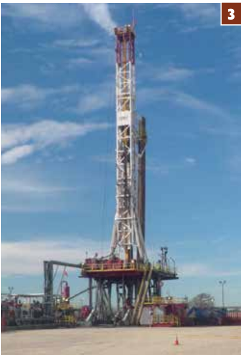
1. For the personless rig floor proof of concept, NOV moved the driller's cabin from the rig floor to the ground below the rig. 2. A combination of well-placed cameras and high-definition screens are giving the drilling engineer a better idea of what's happening with the drilling operation even though the cabin is not on the drilling floor. 3. NOV's test rig in Navasota, Texas, with the driller's cabin on the ground level. NOV tested drilling operations with this set up in December 2023. 4. The video cameras keep an eye on rig floor activity, and the view appears on high-definition screens in the driller's cabin. 5. The rig floor is now a long flight of stairs away from the driller's cabin 6. The drilling engineer can watch the robots perform their tasks. 7. Robots are handling tasks on the drill floor like handling pipe.
