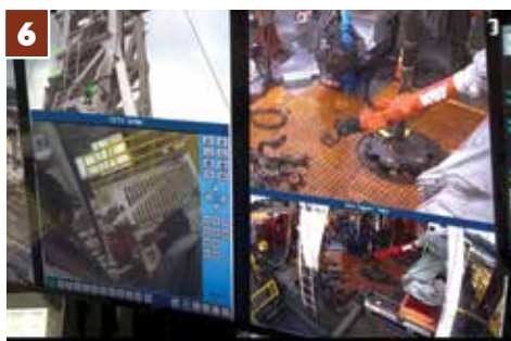
1. For the personless rig floor proof of concept, NOV moved the driller's cabin from the rig floor to the ground below the rig. 2. A combination of well-placed cameras and high-definition screens are giving the drilling engineer a better idea of what's happening with the drilling operation even though the cabin is not on the drilling floor. 3. NOV's test rig in Navasota, Texas, with the driller's cabin on the ground level. NOV tested drilling operations with this set up in December 2023. 4. The video cameras keep an eye on rig floor activity, and the view appears on high-definition screens in the driller's cabin. 5. The rig floor is now a long flight of stairs away from the driller's cabin 6. The drilling engineer can watch the robots perform their tasks. 7. Robots are handling tasks on the drill floor like handling pipe.
