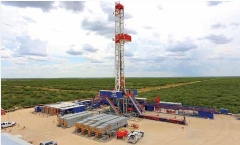
Patterson-UTI's APEX XK drilling rig with walking system.
