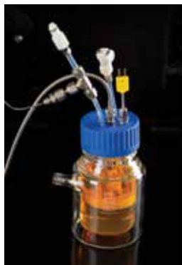
PARA-Window captures paraffin deposition at a more realistic temperature gradient (5°C) between the bulk oil and surface temperature using a near-infrared optical probe.
