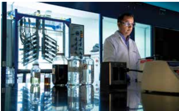
PARA-Window captures paraffin deposition at a more realistic temperature gradient (5°C) between the bulk oil and surface temperature using a near-infrared optical probe.
