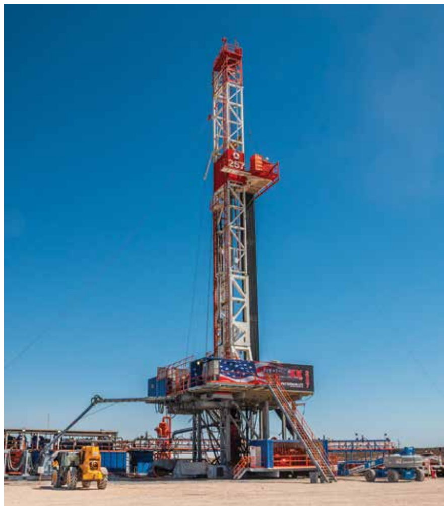
Longer laterals require higher pressures in the drilling process—rising to 7,500 psi today, from just 5,000 psi a few years ago.
