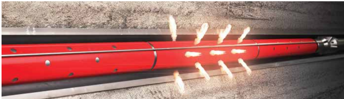
The gun assemblies are oriented so their perforation ports are pointed away from the optical cable, thereby preventing cable or gauge damage before cementing in place.
