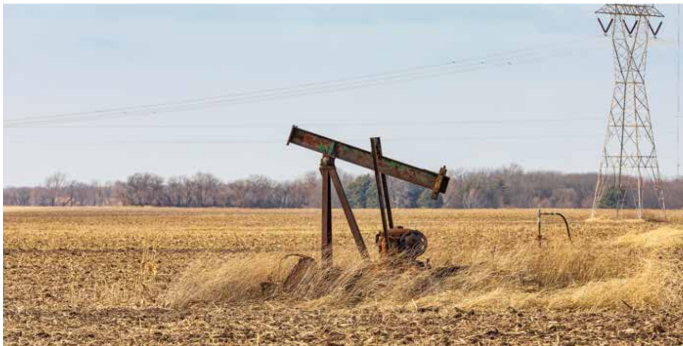
An orphaned well on a farm. Orphan wells are thought to have compromised infrastructure and could become conduits to pollute groundwater if produced water sent into a shallow disposal well migrates into an orphan well.
