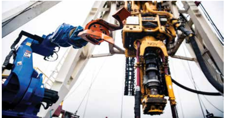
The ATOM RTX robotic system performs tasks including doping, guiding when stabbing, tailing, stand building and mud containment with a high degree of precision and repeatability.
