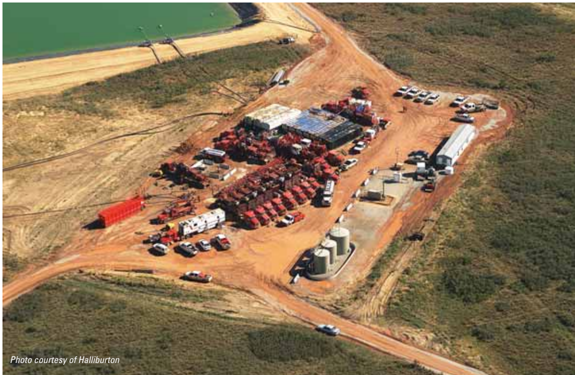
Figure 2. Massive hydraulic frac jobs are required to stimulate multiple stages in the Woodford Shale.
