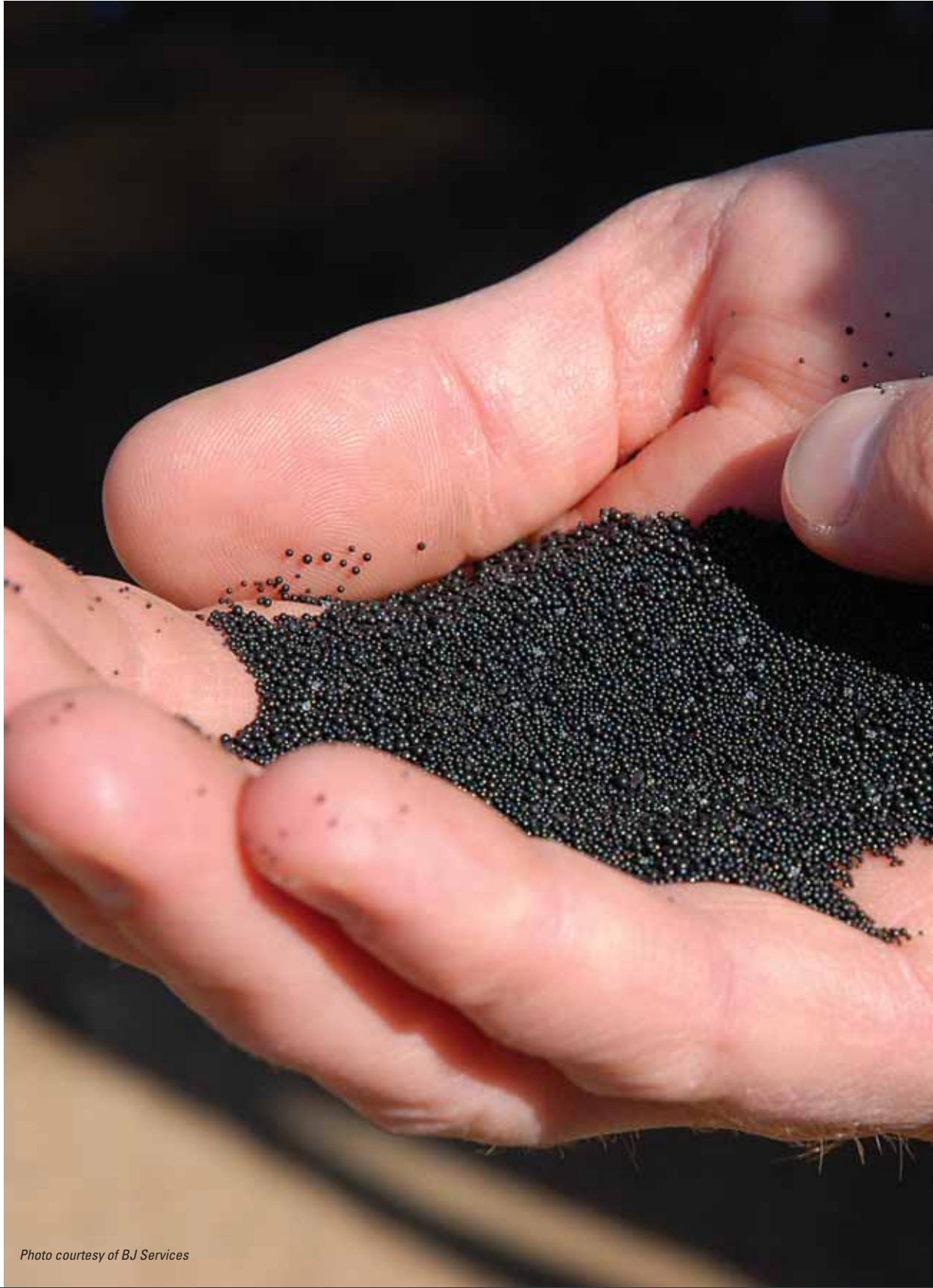
Figure 1. A BJ Services engineer holds a handful of LiteProp beads. The uniform light-weight beads “float” into place in slickwater fracs to extend fracture length.
