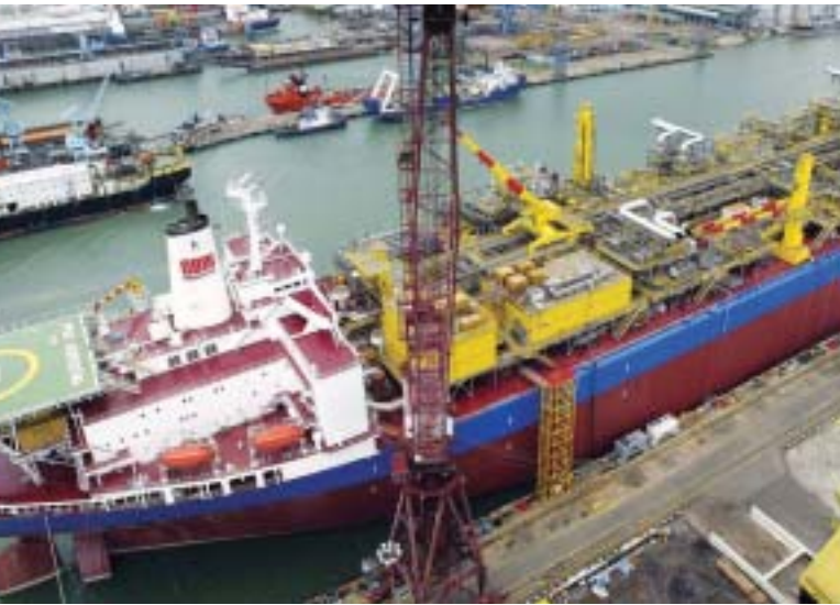
Vessels are converted into floating production, storage and offloading (FPSO) facilities in Singapore.
