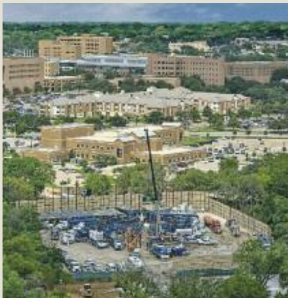
Carrizo rigs up for a massive gas shale frac job at its Barnett properties on the University of Texas properties at Arlington, Texas. Photo courtesy of Carrizo Oil & Gas Inc.
