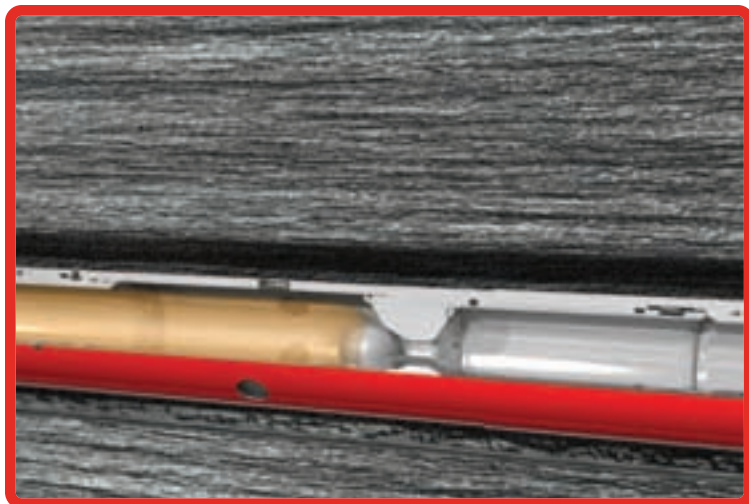
The MASS sleeves system can currently segment a maximum of 10 stages, each consisting of five sleeves in a single installation. (Image courtesy of Weatherford International)
