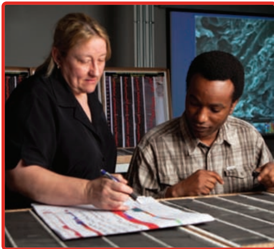
Geoscientists validate a core-to-log correlation for classifying heterogeneous rock types. (Photo courtesy of Schlumberger)
