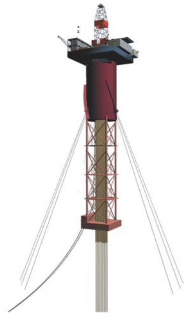
The truss spar provides greater vertical stability over the classic spar.
