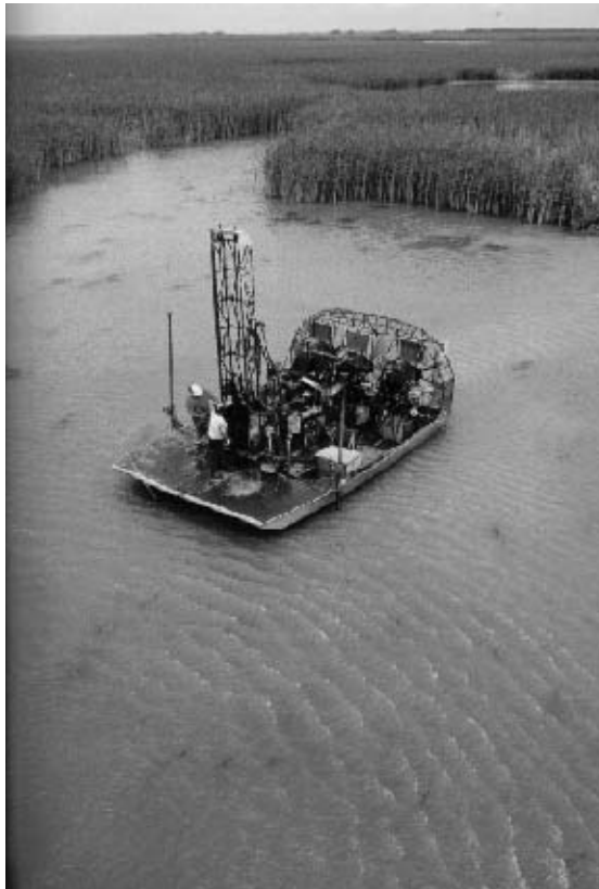
A geophysical crew collects data in the transition zone in Plaquemines Parish, Louisiana, using a shot-hole drill custom-mounted on an airboat.
