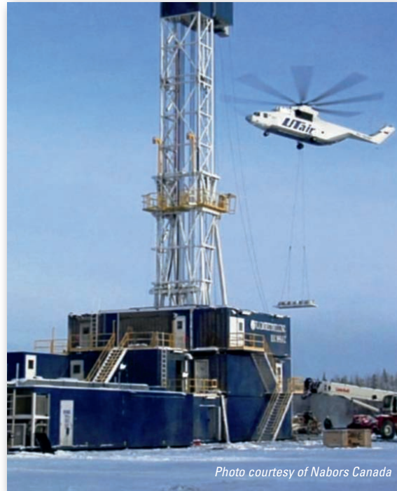
Figure 2. The world's largest-capacity helicopter, the Russian Mi26T, easily transports Nabors Drilling PACE modular electric drilling rig to a remote site in Northeast British Columbia.
