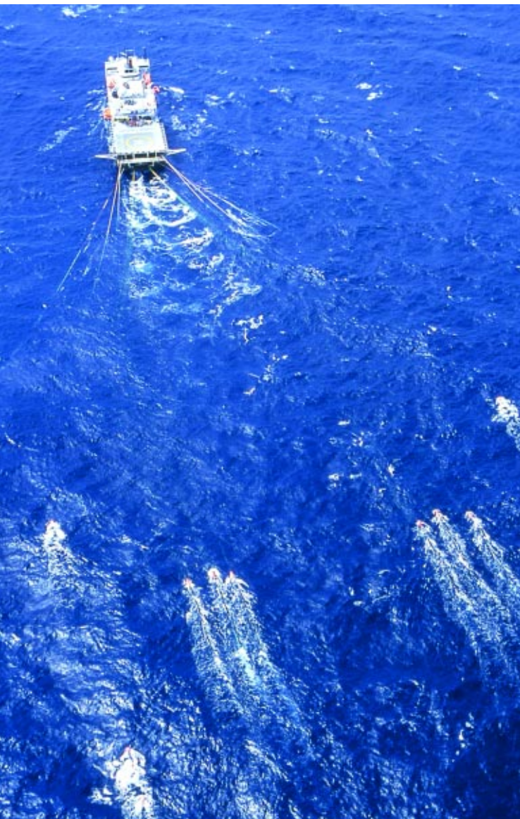
3-D seismic, shown being shot here, helped independents see bright spots of oil and gas in the Gulf of Mexico.
