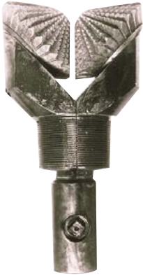
The two-cone bit allowed independents and majors to drill straighter holes faster. (Photo courtesy of Baker Hughes Inc.)
