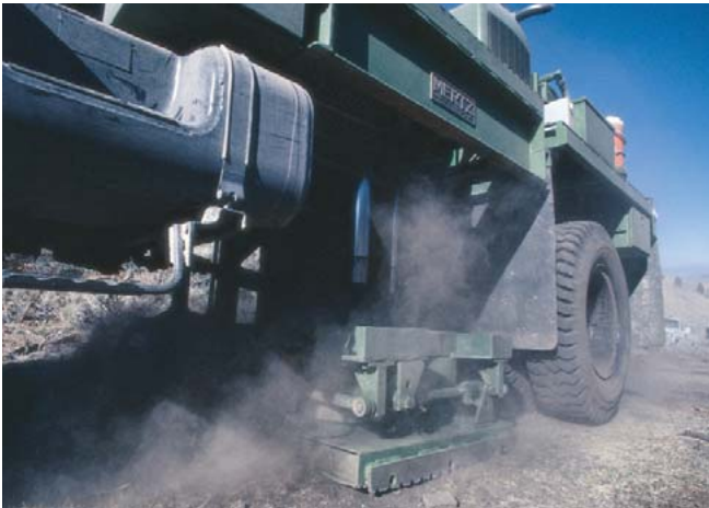
Seismic technology began to be more widely used in the 1950s and 1960s and was credited for Occidental’s oil discovery in Libya, one of the largest oil reservoirs in the world. Conoco scientists developed and patented the Vibroseis method of seismic oil exploration in 1956. (Photo courtesy of ConocoPhillips Corporate Archives)
