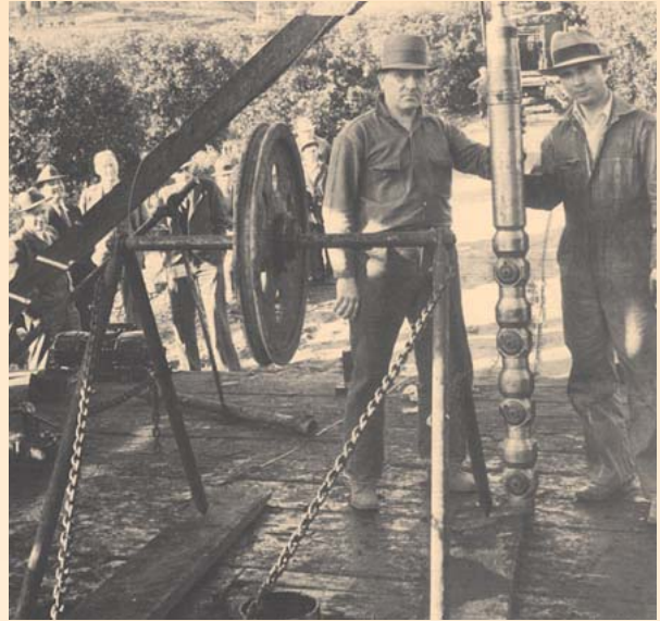
Bill Lane and Walt Wells staked their future on the performance of a perforating gun in 1932 at Union Oil Co.’s La Merced No. 17. (Photo courtesy of From an Idea to an Industry: Fifty Years with Dresser Atlas—1932-1982 )
