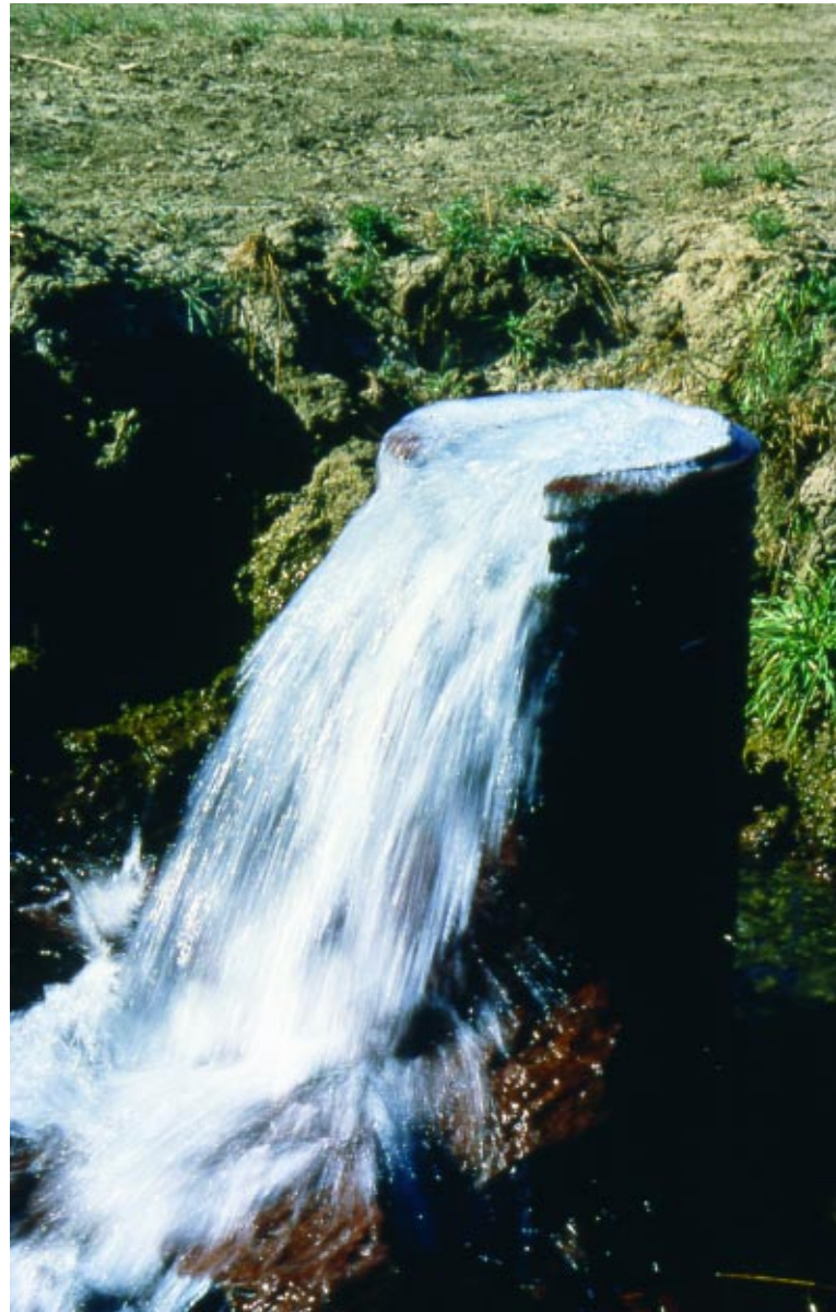
Coalbed-methane wells, made profitable by 1990s economics and technology, produce water for months before gas.
