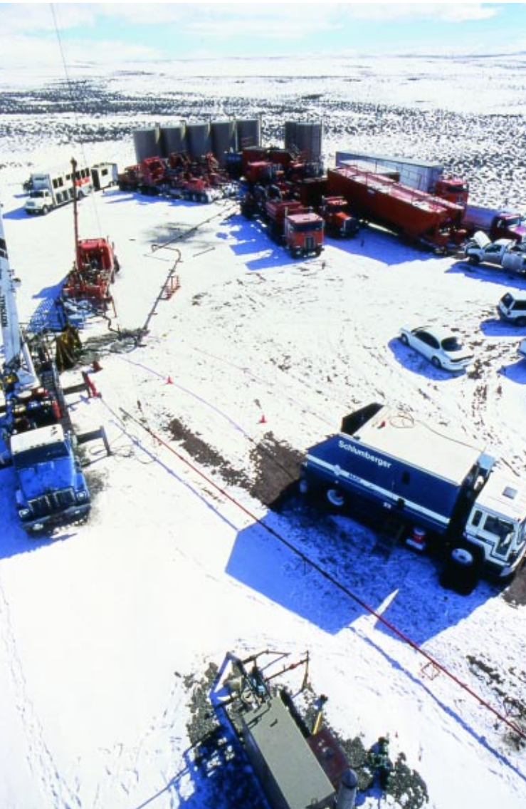
Fracture stimulation improved with computer controls and better proppants in the 1990s. Here, Schlumberger completes a multi-stage frac in Wyoming.
