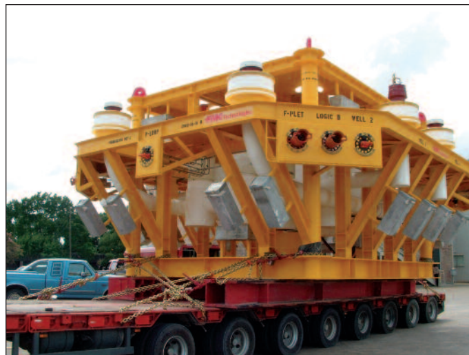
A multi-slot subsea oil and gas manifold with electric and hydraulic controls and automated valves for a field tie-back in the Gulf of Mexico. Subsea manifolds gather flow from multiple wells in working pressures up to 15,000 psi in water depths to 10,000 feet.
