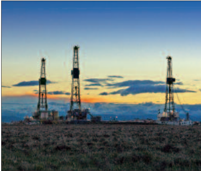
Questar drills multiple wells from a single pad on the Pinedale Anticline in western Wyoming.
