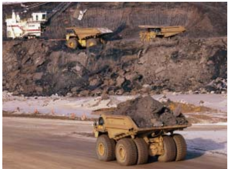
The truck-shovel combination is perfectly matched to optimize efficiency at the mine face as we selectively load from multiple benches within the mine.
