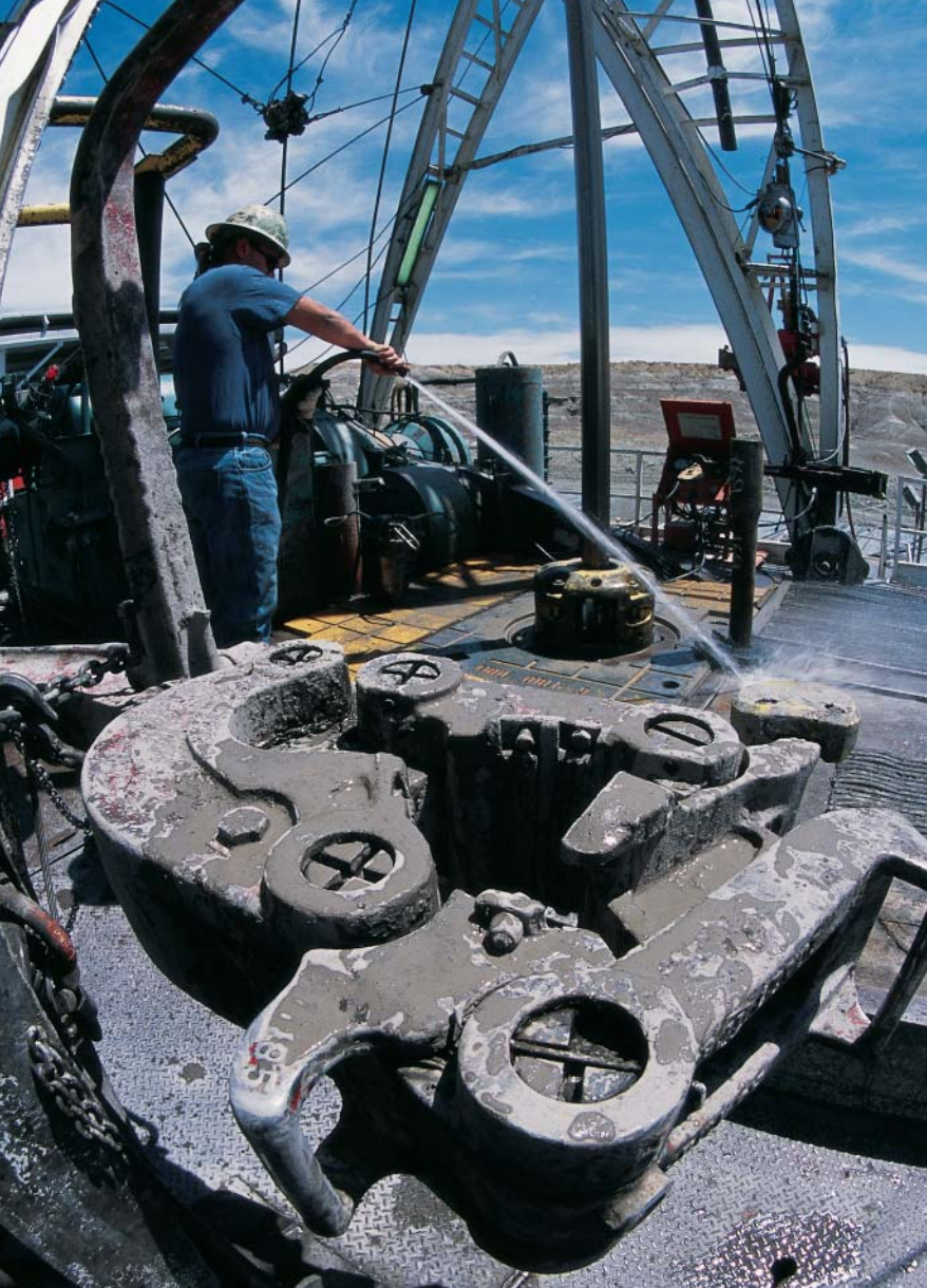
A roughneck cleans the floor of a drilling rig. Shown is the hole, through which the well is drilled, and drilling mud.
