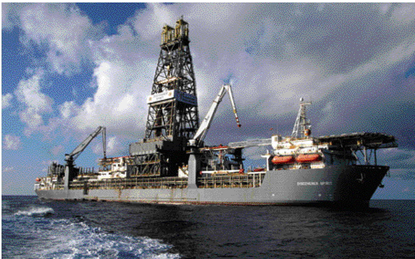
Holder of the world records for ultradeepwater drilling and setting a wet tree in the deepest water depths, the Transocean Deepwater Spirit drillship operates in the Gulf of Mexico under a long-term contract for Unocal Corp. It and two sister rigs—the Discoverer Enterprise and Discoverer Deep Seas —have a patented dual-activity process with two drilling systems in one derrick. Two wells can be drilled or serviced at once.
