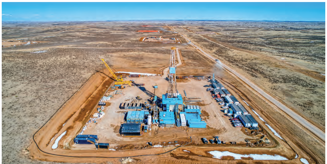
Anschutz Exploration Corp. is currently drilling two Niobrara wells and one Turner well on its multiwell Lucy pad in the Powder River Basin.
