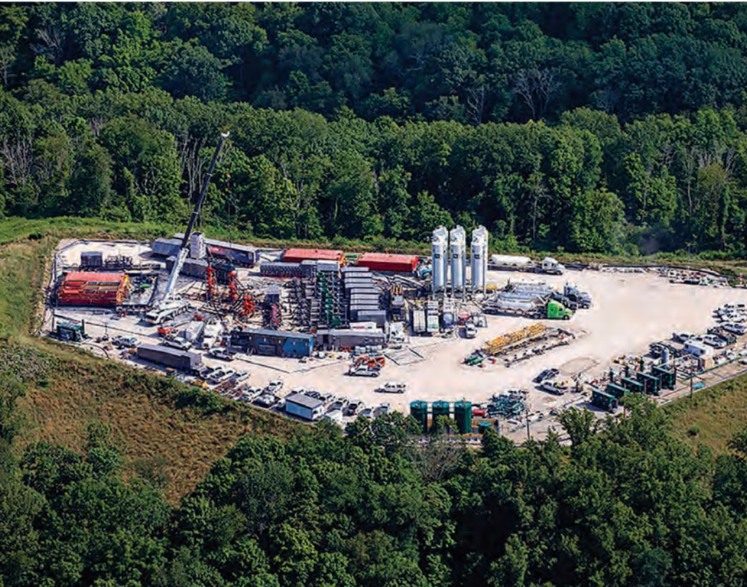
Pictured above and left: Evolution’s electric frac fleets result in zero gallons of diesel consumed during pumping operations, reduced personnel exposure to on site hazards and a 50% smaller footprint than a conventional frac fleet. (Source: Evolution Well Services)
