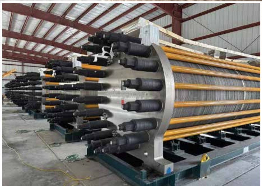
Electrolyzers for the ACES Delta project in Utah.
