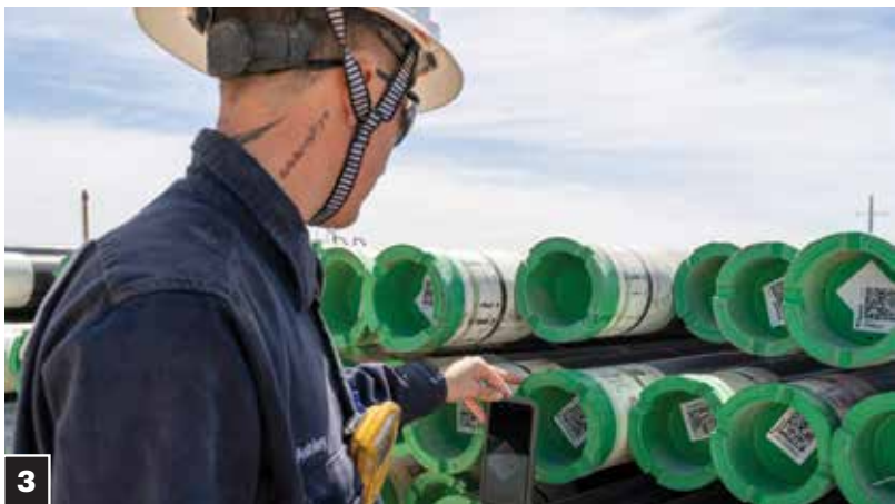
1. Tenaris' Rig Direct tracks pipe from production to installation. 2. The Rig Direct Portal gives clients all their OCTG information in one place, on a cell phone or other smart device. 3. With Tenaris' PipeTracer technology, every pipe is tagged with a unique reference code (URC) that gives clients complete pipe information, including length, weight, the pipe's history and more.
